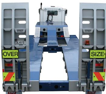
Open centre allows dipper arm to lower below deck
