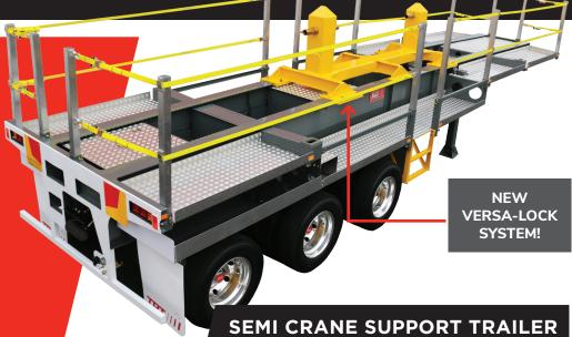
To meet the specialised requirements of the crane industry, we have developed a range of purpose-built lightweight crane support trailers that are designed to securely transport counterweights and other crane components. These are delivered in the right order to be deployed.
