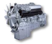
On-highway engines include Series 60, DD13, DD15 and MBE. The metal ID plate on the left hand side (viewed from the flywheel end) of the valve cover shows model and serial number. These numbers are also stamped on the cylinder block just below the intake manifold and above the cast-in Detroit logo. Series 60 serial numbers begin with O6R followed by seven digits.
