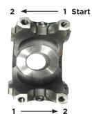
SPL Strap bolts **must** be torqued in the proper sequence. Starting at either position **1** as shown here, torque bolts in an anticlockwise sequence.
