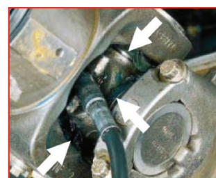
Shaft marked prior to disassembly
