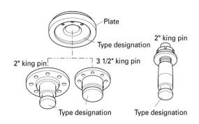
The respective type designation is stamped into the pin and the retention plate: (As shown).
