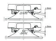
Version C must have a minimum gap of 5mm under load.
