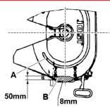
The fifth wheel coupling must be replaced. If the flat top surface is worn to the depth of the lubrication groove (A).
