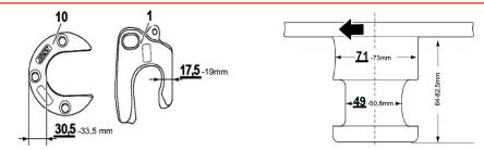
When the wear limit has been reached the affected components must be replaced.
