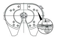
For W models the wear limit of the liners is reached when they have worn down to the top of the securing bolts.
