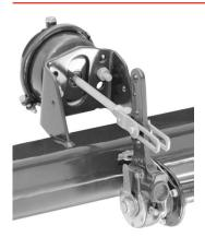
Force from the brake chambers is transmitted by the slack adjuster to the brake camshaft causing it to rotate. The S Cam forces the brake shoes apart, pressing them against the inside of the brake drum. When the brake is released, the brake camshaft rotates the S Cam back to its neutral position.
