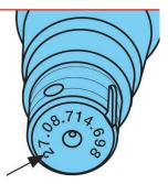
BPW Axle Number punched into the end of the axle stub.
