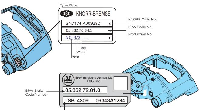
BPW Brake Type & Serial Number of the Brake
