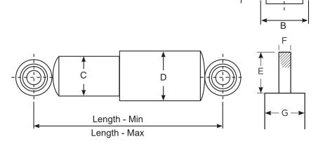
To identify a shock absorber measure length centre line to centre line extended and compressed. Note style of the eye/stud and also the measurements
