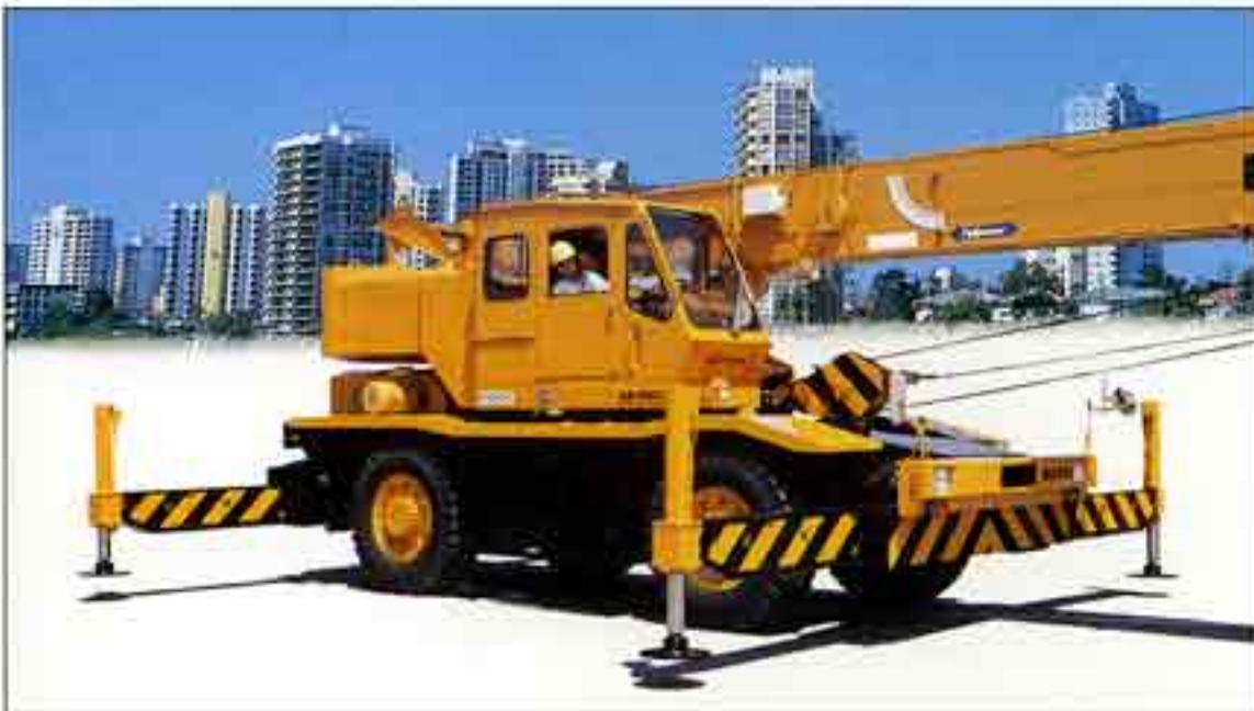
Outriggers can be controllable from operator's cab.
