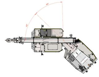
TRT's TIDD PC28-2 is extremely maneuverable, slewing up to 44° working well inside the radius of other pick and carry cranes in its class. At only 2.5m wide the PC28-2 has a smaller foot print, with Slew Safe it's now even safer!
