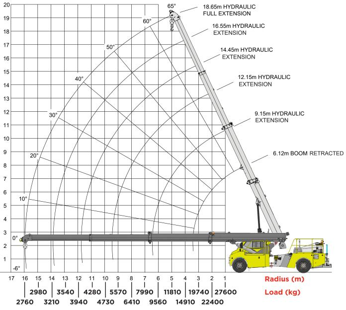
NOTE: Rated capacity values shown are for the stationary chart on the hook.
