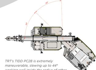
working well inside the radius of other pick and carry cranes in its class. At only 2.5m wide the PC28 has a smaller foot print, with Slew Safe it's now even safer!
