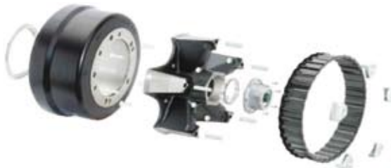
5 Spoke Sider Hub and Drum Assembly
