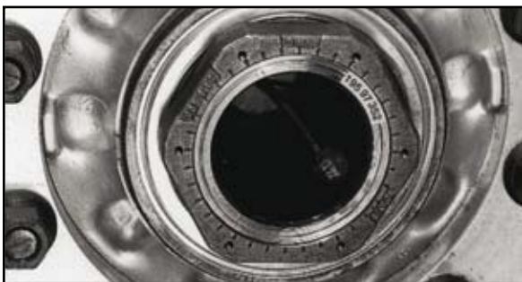
Identification of axles when type plate not available. Production no. of axle on RH side of axle tube.
