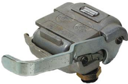
WABCO DUOMATIC AIRLINE COUPLING 452 802 000 0 TRUCK HALF 452 804 001 0 TRAILER HALF
